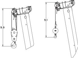
Dimensions are for the largest grove furnished hook block and overhaul ball, with anti-two block activated.
